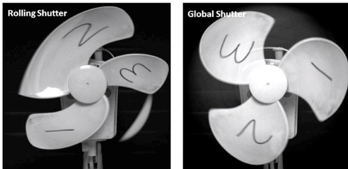
Figure 2 – Images of a moving fan, acquired with Neo sCMOS camera with rolling and global shutter exposure modes, same exposure time. The spatial distortion associated with the ‘rolling shutter effect’ is apparent in the left image. Global shutter is a ‘snapshot’ acquisition mode and avoids spatial distortion.
