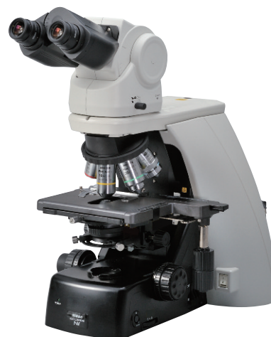
Ni-U configured with ergonomic binocular tube
