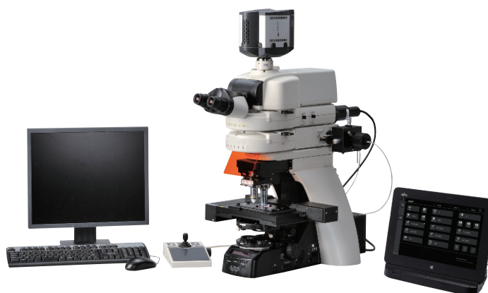
Ni-E (Focusing nosepiece) configured with motorized stage, motorized epi-fluorescence illuminator, photoactivation unit, motorized quadocular tilting tube and camera
