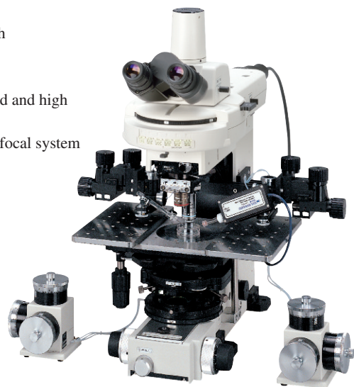
Configuration with Narishige micromanipulators and epi-fluorescence attachment
